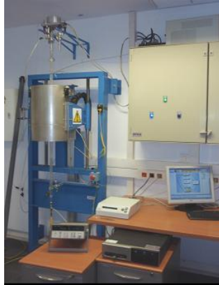
Multicycle testing TG at CSIC
