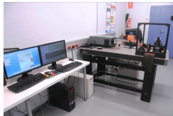
SNOM with high resolution optical spectrometer and an electron multiplier CCD.
